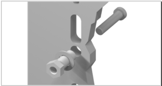
Shank nut/washer through the remote sensor installation plate
