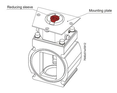
Commission the proportional controlling element only when mounting plate, flange and the respective actuator are correctly assembled.
