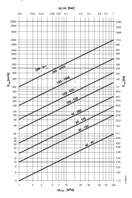
$\Delta P_{v100}$ = Differential pressure across the fully open butterfly valve by a volume flow **V**100
