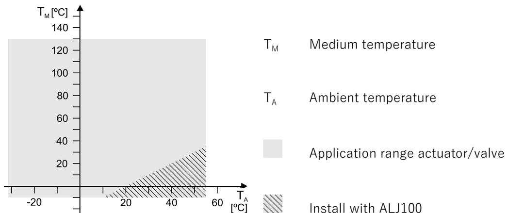
Only use GDB.., GDD..,GSD.. and GQD.. actuators at medium temperatures  $> 0^\circ \text{C}$ .
