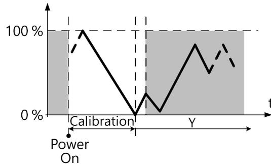
During calibration, the valve is measured and the positions for “valve open” and “valve closed” are stored. In KNX S-Mode, it is possible to only calculate the “valve open” position by working back from a set path from the closed position (to close the valve, the actuator stem extends until the set force is exerted on the valve).
