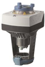
Electromotive actuator to operate Siemens 2-port and 3-port valves, types VVF42..K, VVF42..KC und VXF42.. with 20/40 mm stroke, as control and safety shutoff valves on heating, ventilation, and air conditioning plants.
