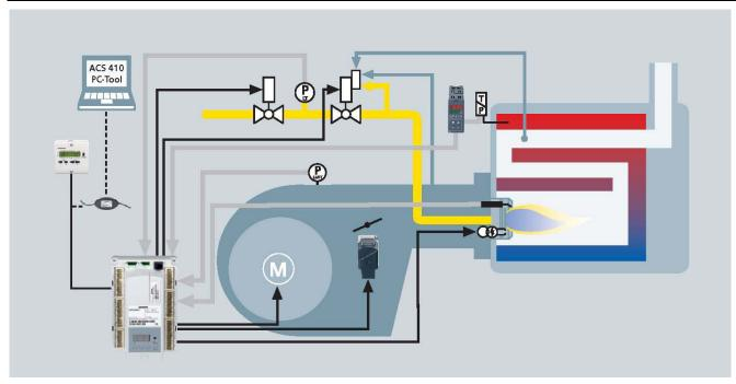
The diagram shows the maximum functionality of the LME7. The actual functions are to be determined based on the respective execution or configuration.
