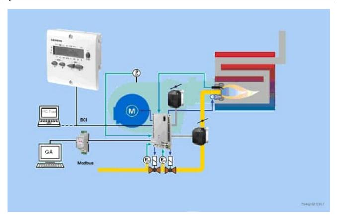
The diagram shows the full scope of functions of the LMV27. The actual functions are to be determined based on the respective execution / configuration!
