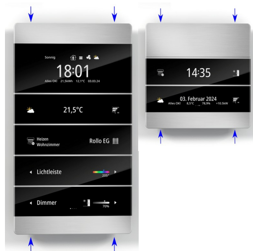
Figure 2: Screwing the MeTa 2 KNX unit to the mounting plate
