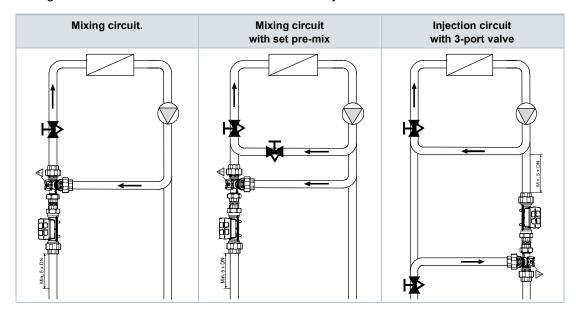
An unhindered inlet section of  $L \ge 5$  x DN must be maintained upstream of the flow sensor to guarantee the indicated measurement and control accuracy.
