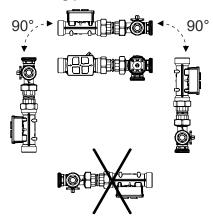
Mount the flow sensor in the return if the media temperatures exceed (>90 °C). If not possible, mount the Intelligent Valve controller remotely from the flow sensor and use the wall-mount plate EZU-WA.
