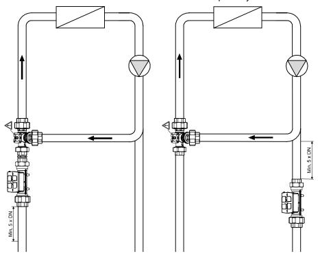
The Intelligent Valve is assembled at the mounting location. No adjustments, with the exception of configuring with the ABT Go app (see Commissioning [ $\rightarrow$  22]) nor special tools are required. Separate mounting instructions are included with the valve and flow sensor.
