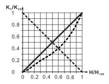
The characteristic curve in the through-port is linear (\_ \_ \_ \_ \_ ).
