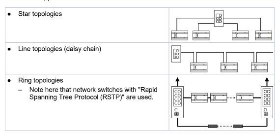
In the case of a daisy chain, it is recommended not to use more than 10 devices per chain. A complete list of supported BACnet data points is included in the document "Intelligent Valve – BACnet Objects" (Product documentation [→ 15]).
