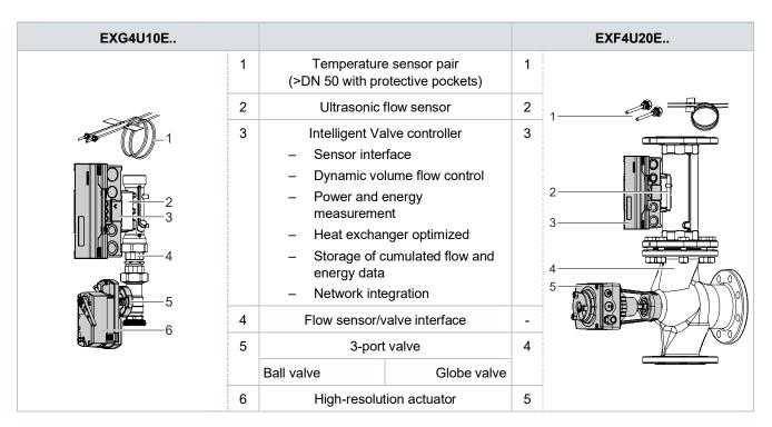
Volume flow is acquired continuously in the ultrasonic flow sensor and provided to the Intelligent Valve controller, where the controller applies it as the actual value for control or limitation by guiding the control valve position until the volume flow actual value for the applicable setpoint is achieved.
