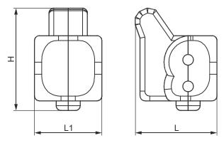
H = Total height of valve with insulation shell to wall or ceiling, for mounting, connection, operation, maintenance etc.
