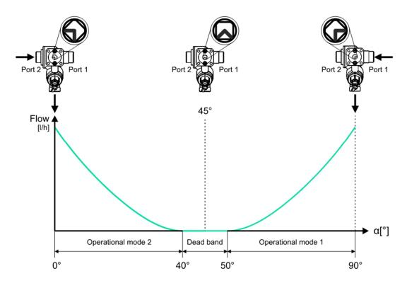
Note that the valve angle  $\alpha$  [°] moves counter-clockwise (CCW). The GDB161.9../..6.. actuators' default rotation direction is CCW, therefore:
