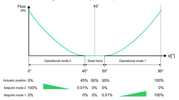
Cooling and heating allocation is freely selectable. However, Siemens suggests an equal allocation for all valves during installation for safety reason as below:
