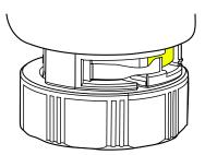
The movement and actual position of the actuator stem is indicated by the yellow stroke indicator.
